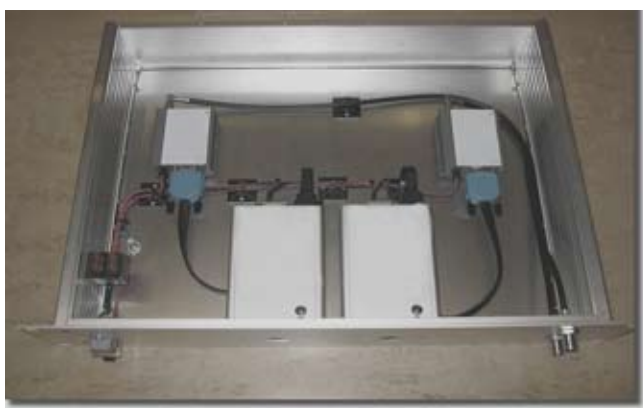
Figure 12. Two GSM modules combined with RoIP Interface Units to create an interconnect from a two-way radio network to a GSM cellular network (provides two independent phone channels) This example is used in a command and control vehicle.
