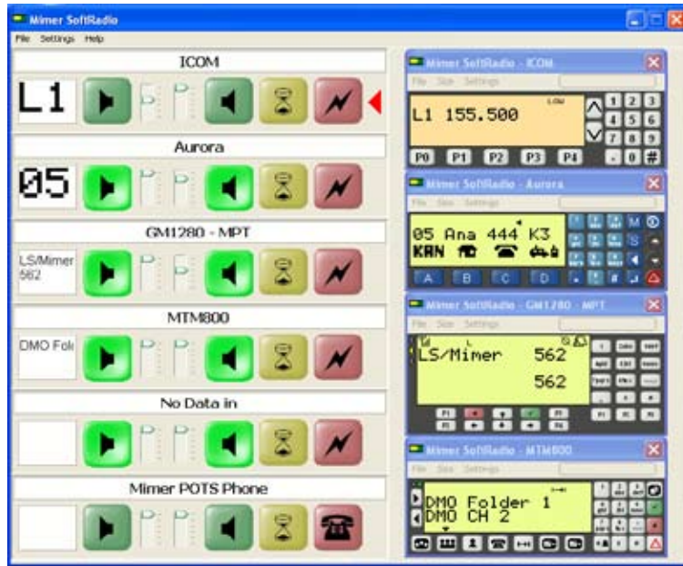
Figure 2. Basic SoftRadio Operator Interface with active Virtual Control Heads
