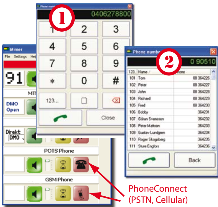
Figure 12. SoftRadio PhoneConnect add-on with dial-pad and speed-dial pop-up windows
