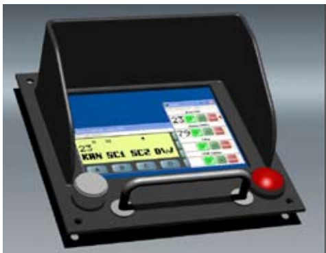
Figure 16. SoftRadio on touch screen PC for installation in a control panel (used in Command & Control vehicles)
