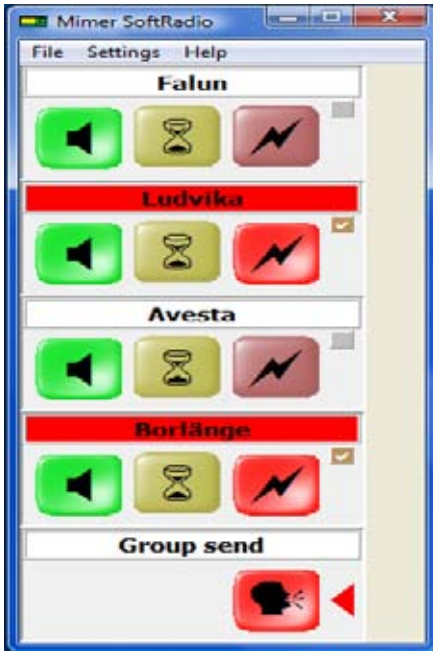
Figure 11. SoftRadio GroupSend add-on and configuration (SoftRadio with four radios, two configured for GroupSend)
