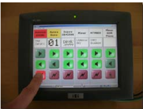
Figure 15. SoftRadio console on touch screen PC
