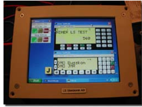
Figure 16. SoftRadio on touch screen PC for installation in a control panel (used in Command & Control vehicles)
